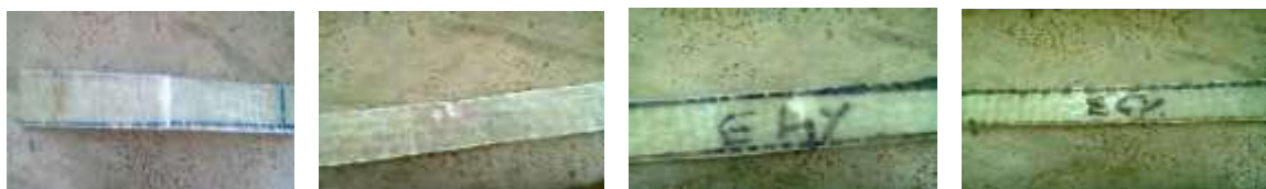
0% filled bending specimen 2% filled bending specimen 4% filled bending specimen 6% filled bending specimen Fig (3.2.a) De-lamination of fibers due to bending load
